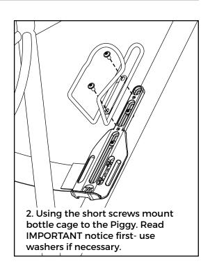
The use of side access bottle cages may be necessary for some frame designs.
