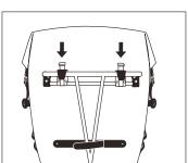
${\bf 3}$   ${\bf \&}$   ${\bf 4.}$  Press the grey buttons to lock the pannier to the rack.
