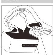
**2.** Pass the Velcro strap through the metal loop.
