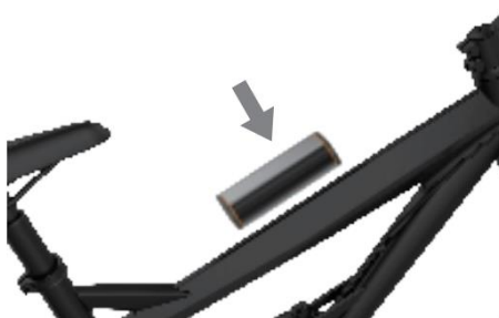
① Secure the battery pack on the frame.
